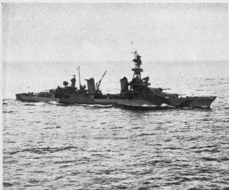
U.S.S. Pensacola rebuilt has solid control tower instead of the old stump mainmast and lower AA and searchlight platforms replacing blocky tower aft of the second stack. Pensacolas have little freeboard.
